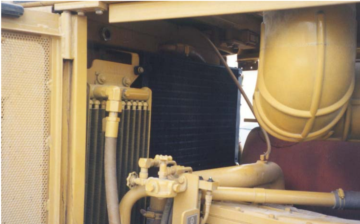
Left side of condenser assembly.
